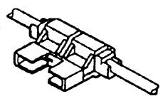
twist the wire to get it to go into the hole. Then take the piece on the top right (with the metal in it) and fold it toward the wire until it contacts the wire. Use pliers to squeeze it down until the latch catches. Repeat this for the wire on the other side. This creates an inline fuse holder.
