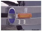
out of bracket hole. Side signal light over clamp stud. Put assembly back into bumper bracket hole, sandwiching signal light between bracket and bumper assembly. Reassemble bumper clamp and tighten firmly.
