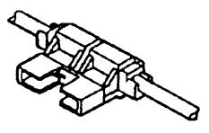
to get it to go into the hole. Then take the piece on the top right (with the metal in it) and fold it toward the wire until it contacts the wire. Use pliers to squeeze it down until the latch catches. Repeat this for the wire on the other side. This creates an inline fuse holder.
